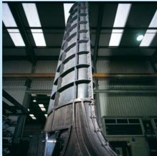
Specialist formwork is manufactured to create an impressive light structure
